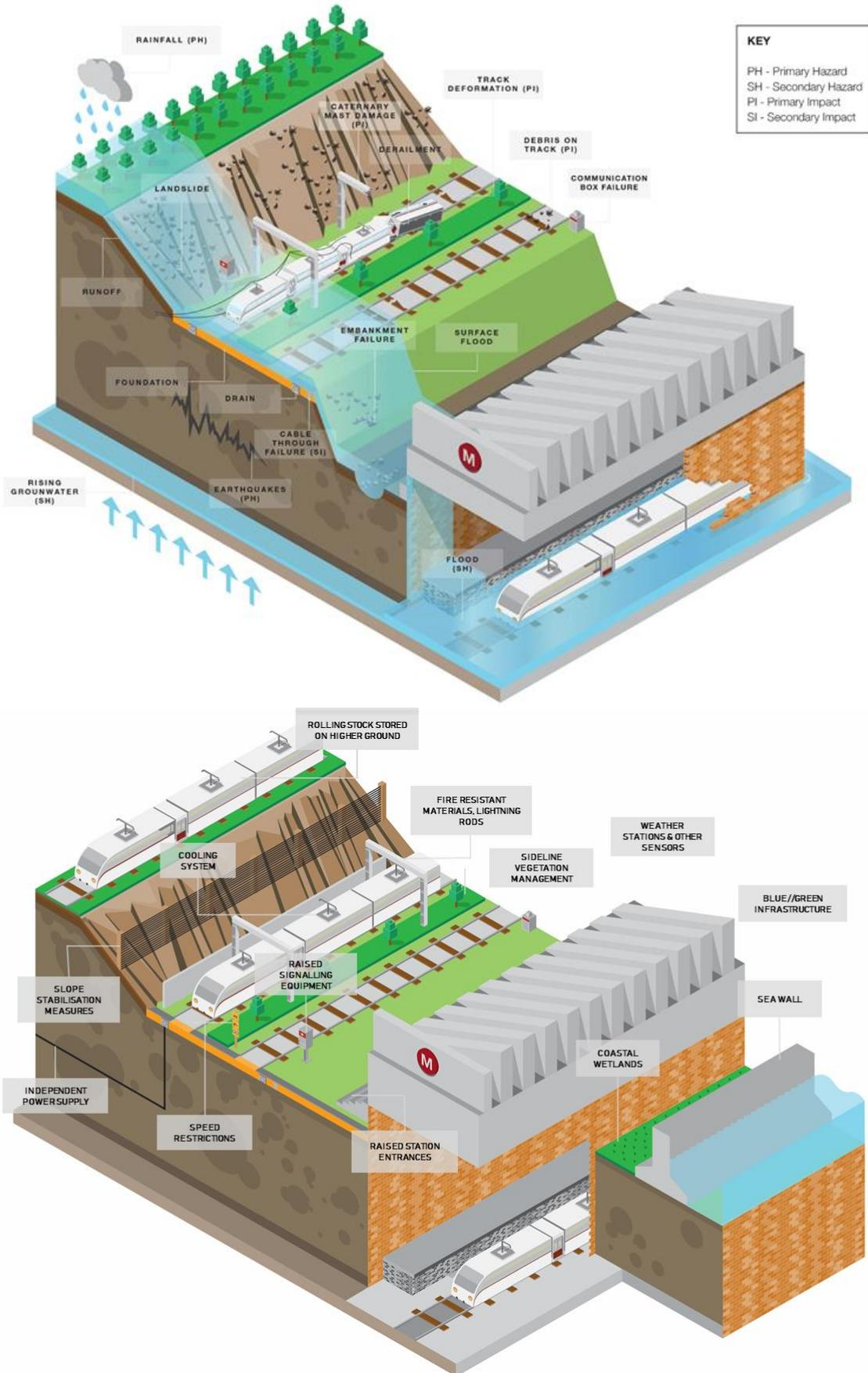
Fig. 3 Graphical representation of natural and climate hazards that can have an adverse impacts on urban rail and examples of prevention/mitigation measures (© Arup)
